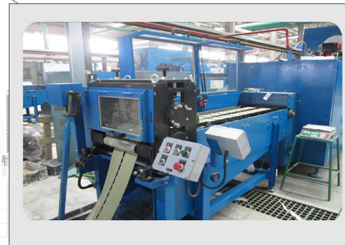
Continuous pasting production line
